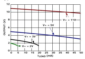
FIGURE 9. COMPARATOR OUTPUT HIGH VOLTAGE vs LOAD
