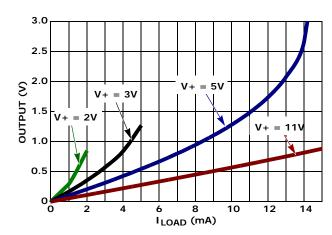
FIGURE 8. COMPARATOR OUTPUT LOW VOLTAGE vs LOAD
