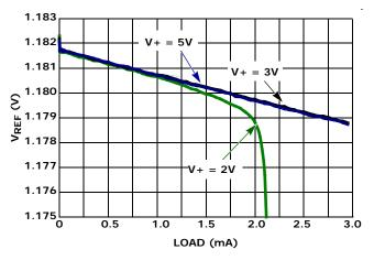
FIGURE 5. V<sub>REF</sub> vs LOAD (SOURCE)
