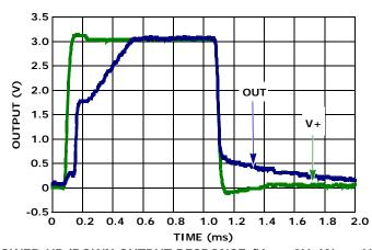
FIGURE 23. POWER-UP/DOWN OUTPUT RESPONSE (V+ = 3V, IN+ = V+, IN- = V<sub>REF</sub>)
