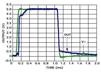
FIGURE 22. POWER-UP/DOWN OUTPUT RESPONSE  $(V + = 5V, IN + = V +, IN - = V_{RFF})$
