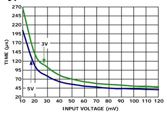
FIGURE 21. OUTPUT RESPONSE TIME vs INPUT OVERDRIVE (tplH)
