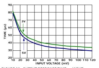
FIGURE 20. OUTPUT RESPONSE TIME vs INPUT OVERDRIVE  $(t_{PHL})$
