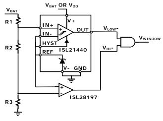
FIGURE 25. WINDOW COMPARATOR CIRCUIT
