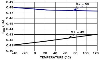
FIGURE 1. I<sub>DD</sub> vs TEMPERATURE
