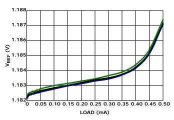
FIGURE 6. V<sub>REF</sub> vs LOAD (SINK)
