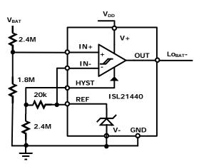
FIGURE 24. LOW BATTERY DETECTOR WITH HYSTERESIS
